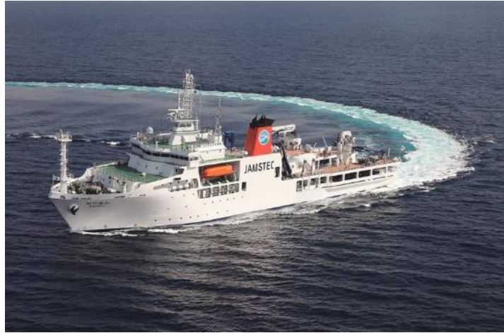
Kaimei Built: 2016 L×B: 100.5×20.5 (m) Gross tonnage: 5,747 Accommodation: 65 (38) (for researcher) Main objective: Subseafloor research
