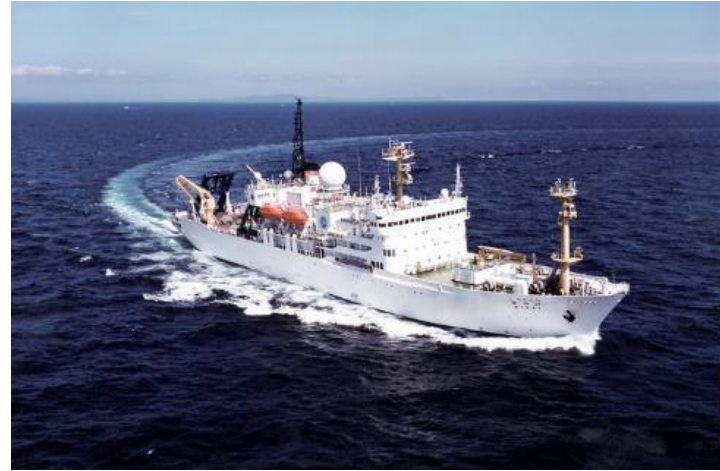
Mirai Built: 1997 L×B: 128.5×19.0 (m) Gross tonnage: 8,706 Accommodation: 80 (46) (for researcher) Main objective: Atmospheric and Oceanographic research
