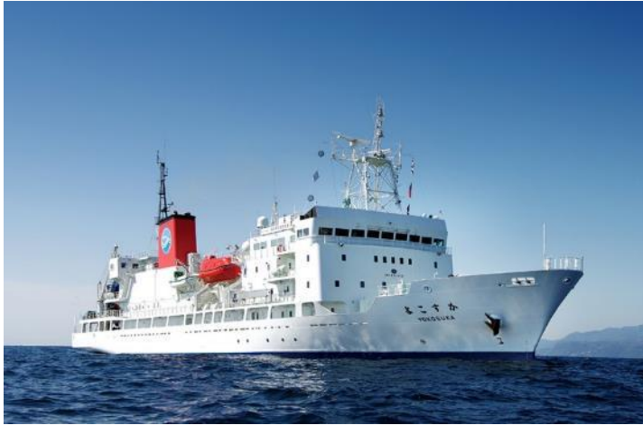
Yokosuka Built: 1990 L×B: 105.2×16.0 (m) Gross tonnage: 4,439 Accommodation: 60 (15) (for researcher) Main objective: Deepsea research
