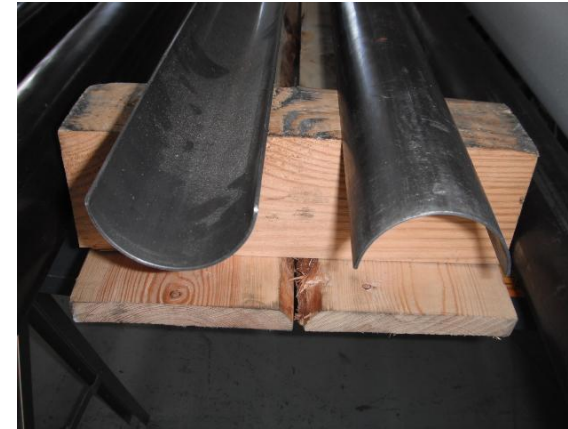
○ Split steel core liner : \Phi 66 \times 61.1\text{mm} 1537mm
