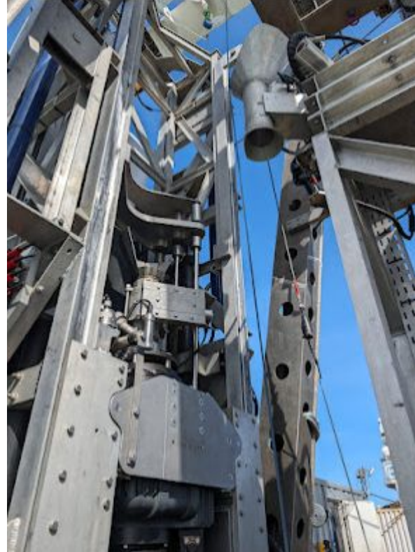
Drill motor moves up and down on tracks
