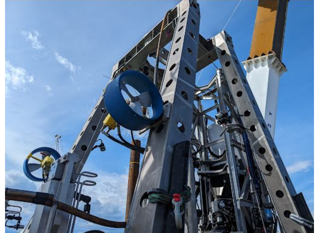
Thrusters for orientation when landing
