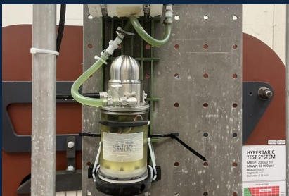
Harmonic Servo Pressure testing
