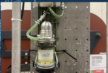
Harmonic Servo Pressure testing
