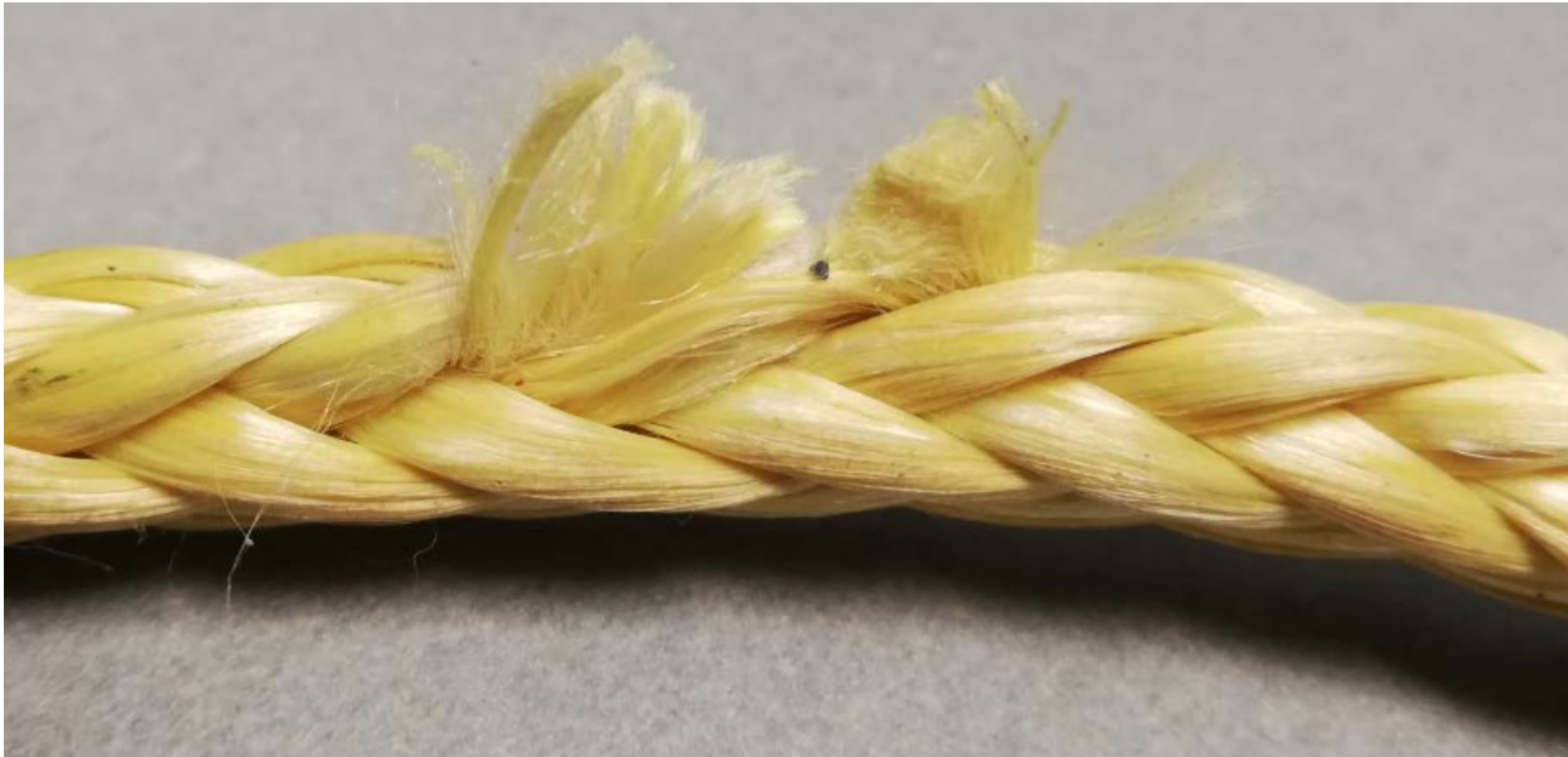
Partially cut strand
