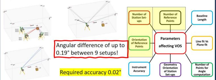
Having more reference points, number of station setups, and verity of orientations provides redundancy and helps identify/minimize/reduce the absolute error.
