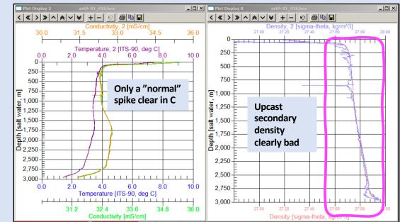
• The upcast density clearly highlights the secondary sensor suite as being impacted by the contamination event.
