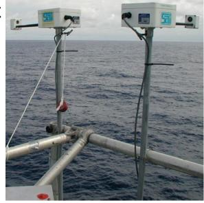
Rain gauges located on the aft part of the ship may overestimate by catching water that has accumulated on the superstructure.
