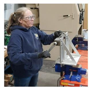
1/4", 3/8", 9/16" 3 x 19 Wire Rope Mandrel Wrap Test
