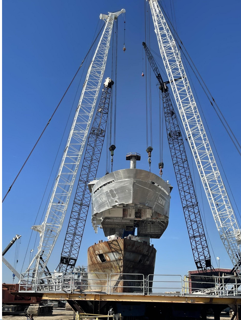
Aluminum superstructure erected onto hull Super Module 10/31/22.
