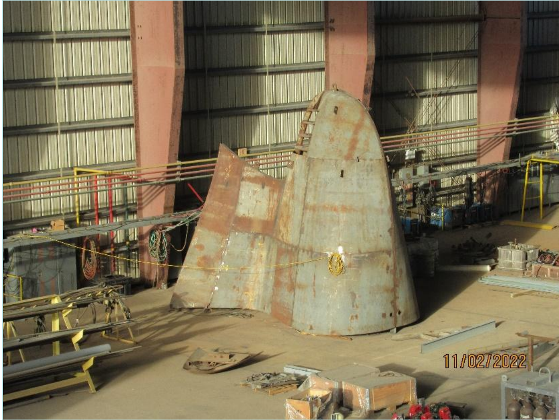
Module 21 adding shell plate
