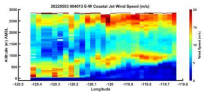
TODWL wind measurements: Illustrates how the NE down slope flow from land to water is undercutting and lifting the low level jet over the Santa Barbara Channel (courtesy of D. Emmitt)
