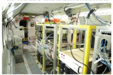
**Cabin**: Nephelometer, Sootphotometer, CPCs, UFCPC, Data System Racks for 'Research' and 'Guest' Instruments. Satcom system
