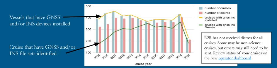
All vessels have GNSS and/or INS systems installed, but raw data is not always logged or identified in the directory structure. All cruises that collect data should log full resolution, raw navigation. Be sure R2R knows how to find your primary, for-science navigation data within the cruise distro.
