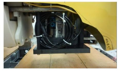
Fornari 20mpx camera installed aft end of Sentry
