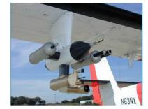
**Wings**: CAPS, FSSP, PCASP, CIP, PIP ... Hard points and pods for 'research' or 'quest' instruments
