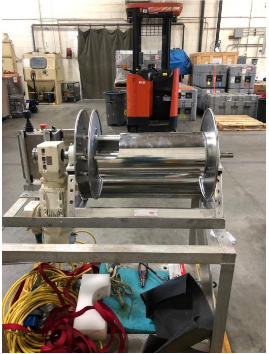
Refurbished magnetometer winch (1 of 2) for SeaSpy 1 and 2 maggie systems
