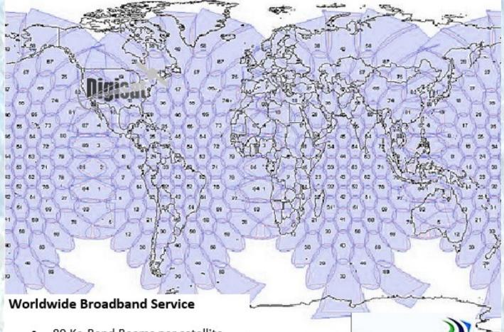
89 Ka-Band Beams per satellite
