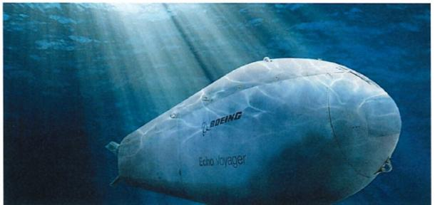
autonomous diesel-electric submarine that has demonstrated a top speed of 9 knots and capability to dive to 11,000' depth.
