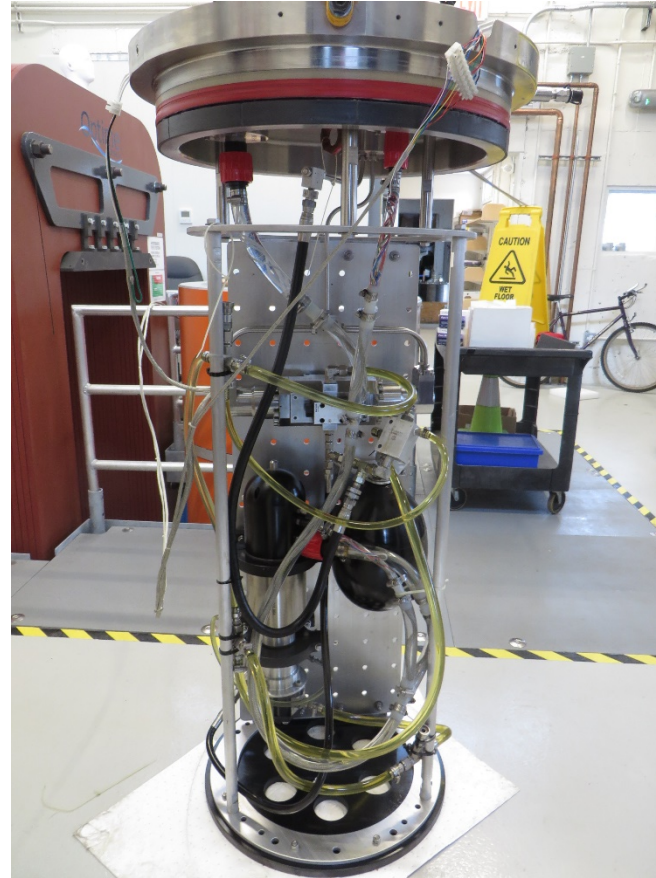
Seawater Pump Test Frame
