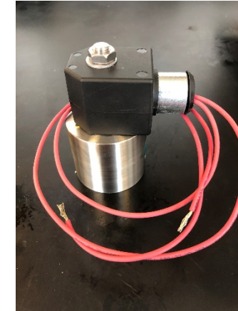
Main Ballast Blow Valve
