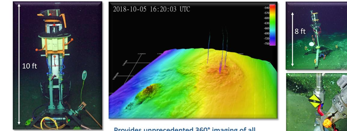
Multibeam sonar, 700 m range, every 2 hrs for ~ 12 minutes Provides unprecedented 360° imaging of all methane plumes issuing from SHR. First flux measurements.
