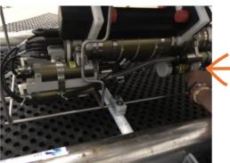
Figure 3. Example of how NOT to install the FLBB. Instrument is not facing free water which resulted in artificially elevated scattering values.
