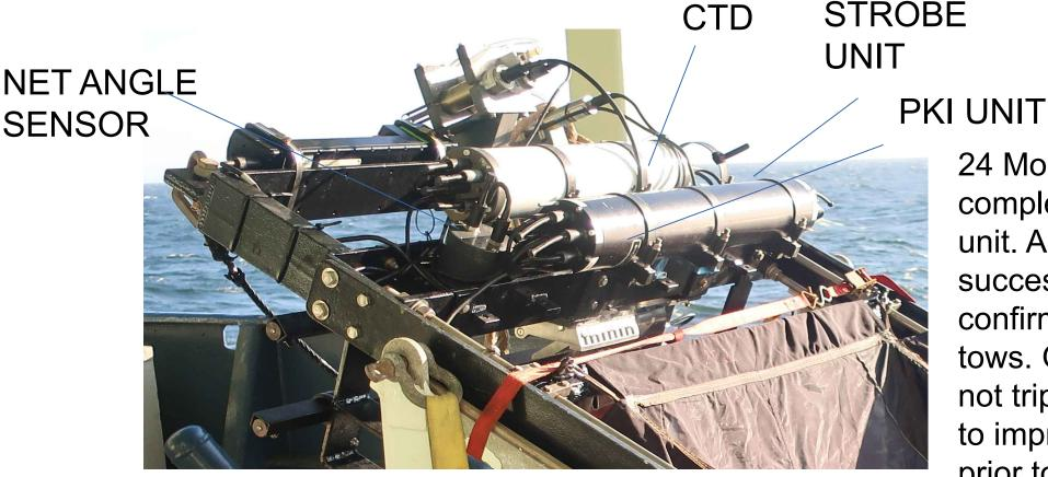
24 Mocness tows were completed using the PKI unit. All Nets were successfully tripped and confirmed on 23 of the tows. On the tow that did not trip/confirm it was due to improper Net preparation prior to the tow.
