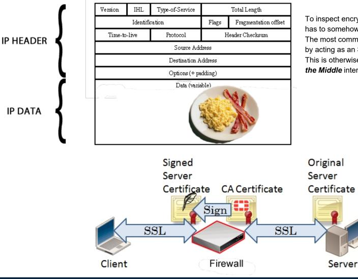
To inspect encrypted traffic the router has to somehow decrypt the IP data. The most common way of doing this is by acting as an SSL Certificate Proxy. This is otherwise known as a *Man in the Middle* interception.
