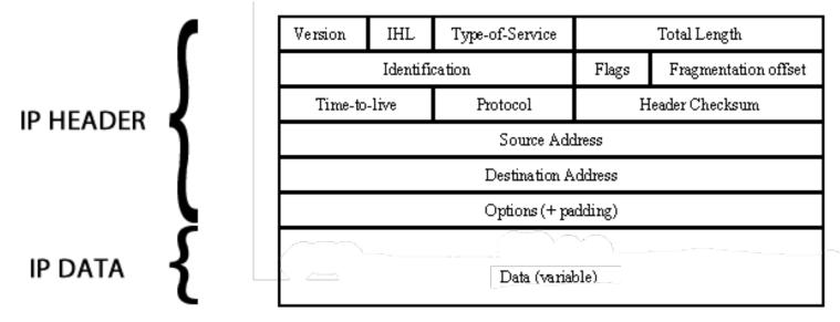
DEEP PACKET INSPECTION, as the name implies, allows the router to inspect the IP data to make routing decisions and perform other higher level functions. Most modern routers and all network security devices perform some level of DPI.
