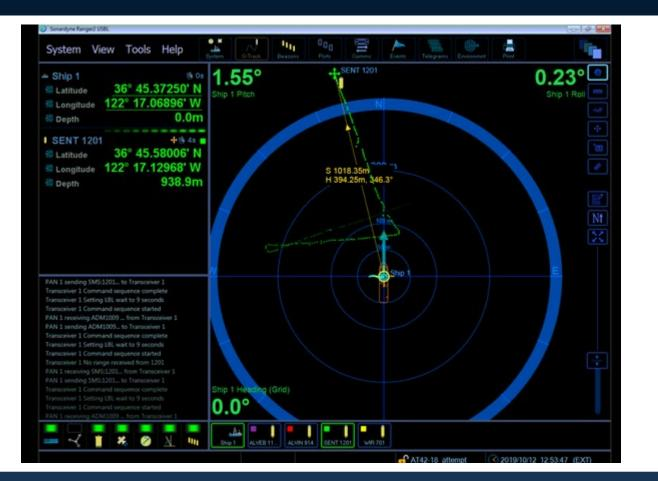
USBL is used within the NDSF facility for range, bearing, and acoustic communications with the three vehicles in the facility (Alvin/Jason/Sentry). NDSF moved to USBL ~ 2009 moving away from LBL transponder nets. This significantly reduced setup time once on station, removing the need to deploy and survey LBL transponders.
