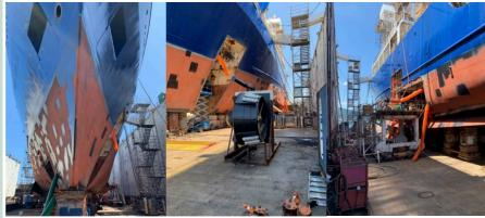
Hull with openings for thruster and engine install, one coat of A/C paint
