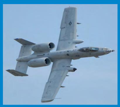
A-10 has 11 hard points on wings and belly where 8000 lbs of instruments may be suspended.
