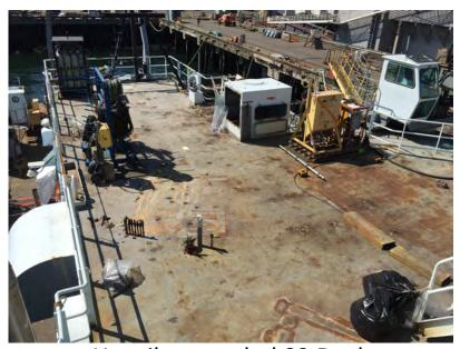
Heavily corroded 02 Deck
