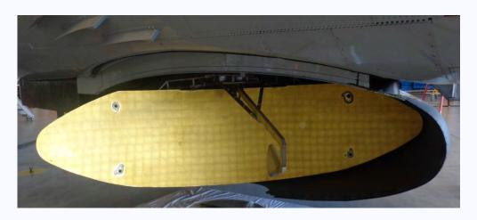
Replace Lower Fuselage Weather Radar with AN/ APY-11 Multimode Radar System
