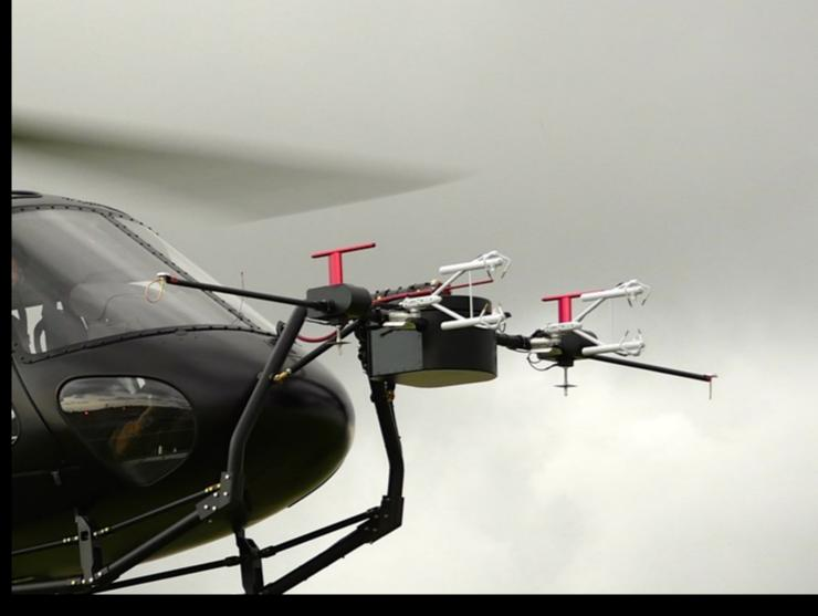
The University of Miami **Helicopter Observation Platform** (HOP) equipped with its Quadruple Eddy Covariance System (QECS) for the detection of gravity waves and turbulence fluxes Hurricane Irma 2D field of gravity waves simulated at 2,000 m MSL with the University of Miami Ocean-Land-Atmosphere Model (OLAM)
