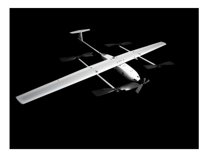
Wingspan 12' Length 7' Weight 24 lbs Payload 5.5 lbs Speed 30(-39) knots Comms range 32 nmi Aircraft range 200 nmi All-weather ops Hand, rail, Bungee or VTOL launch Glide or VTOL recovery Range dependent on battery/ops choices: 1 - battery only = 2 hours for VTOL, 4 hr forhorizontal flight 2 – propane fuel cell = 8 hours They tend to not use VTOL for launch/recovery because of battery use, but for ships would be best.
