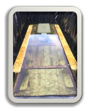
Figure 3: A view inside the test tank. The two concrete blocks (centre, top) were used for the drill testing. . The smaller block had several seafloor rocks interspersed in the concrete.
