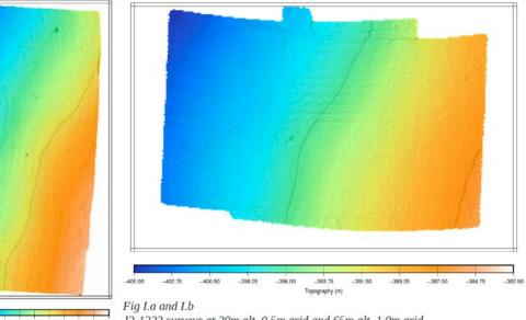
J2-1223 surveys at 20m alt, 0.5m grid and 65m alt, 1.0m grid 403.75-402.50-401.25-400.00-398.75-397.50-396.25-395.00-393.75-392.50-391.2 Topography (m)
