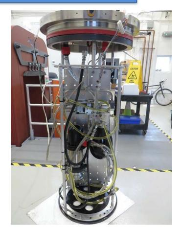
Seawater Pump Test Frame
