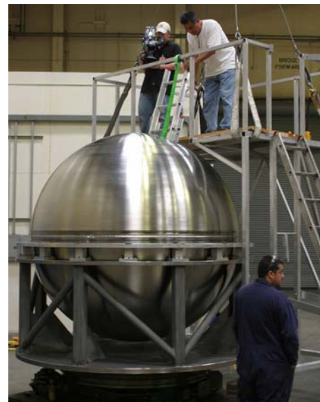
Figure 3. The titanium personnel sphere after electron beam welding of the two hemispheres in August 2009. (Image courtesy of Matthew Blute, Open Road Pictures and WHOI).
