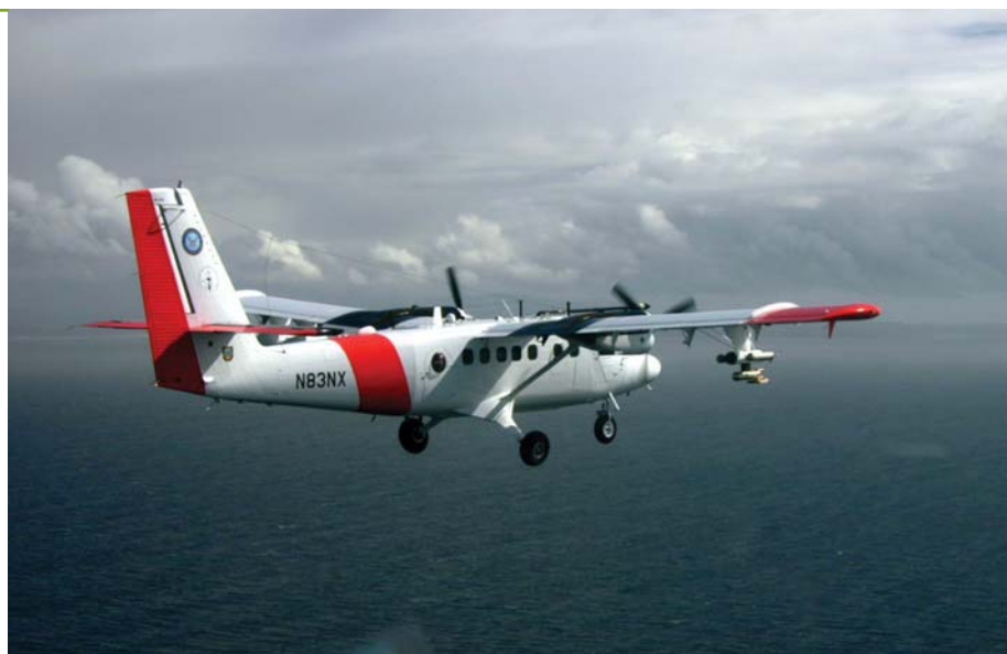
Figure 5. The UV-18A Twin Otter turboprop aircraft operated by the Center for Interdisciplinary Remotely-Piloted Aircraft Studies for oceanographic and meteorological research. Important operational characteristics of this aircraft include: Maximum endurance of 8 hrs (extended further during ferry operations), maximum altitude of 25,000 ft, 70-160 knots operational speed range, 200 amps of payload power (DC and AC combined), wing span of 65 ft, gross takeoff weight of 13,500 lbs, and an approximate 6,000 lbs useful load.
