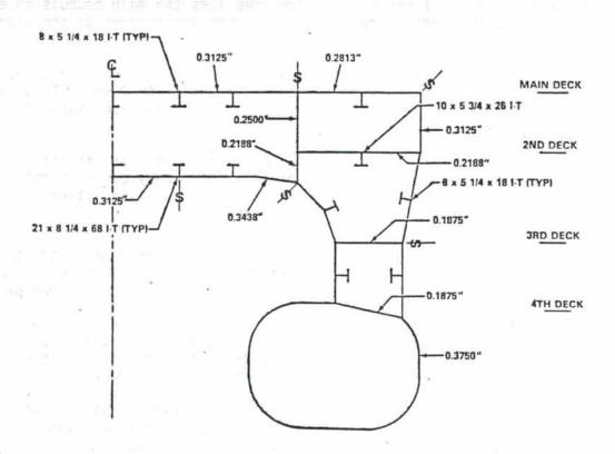
Figure 4.2. Midship Section of SWATH Structure
