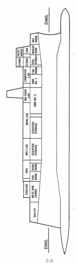
Figure 4.1. Baseline SWATH Inboard Profile
