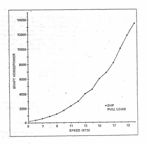
Figure 4.3. Speed/Power Curve AG(X) SWATH
