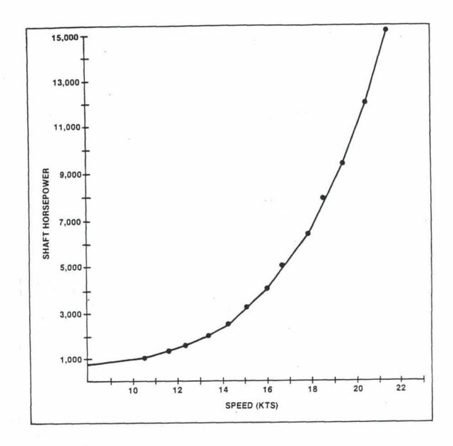
Figure 3.3. Speed/Power Curve for AG(X) Monohull
