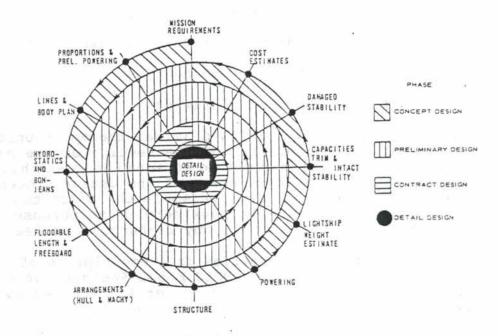
From Ship Design and Construction, Society of Naval Architects and Marine Engineers, 1980
