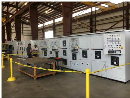
New switchboards undergoing Factory Testing
