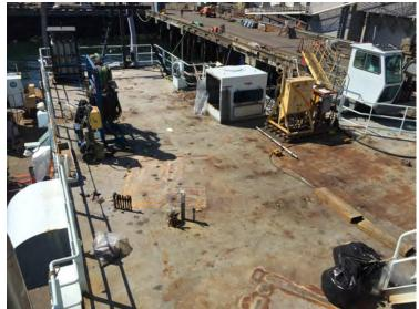
Some deck plating replacement, new paint, new hydroboom foundation, updated hydro-winches & new foundations
