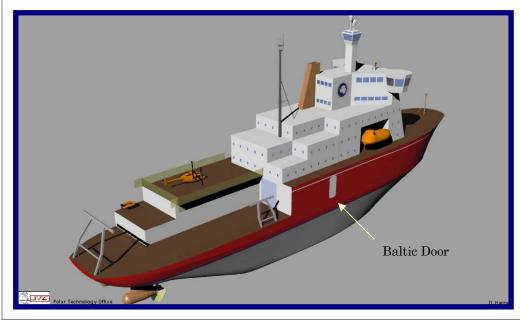
PALMER (NBP). There is also a need to deploy in landfast ice including old ice found in some bays of Antarctica. These requirements necessitated a hull and propulsion plant capable of operating in multiyear ice. As a result, the PRV will also have the capability to operate independently in Arctic ice along the coastal shelf and into the Arctic Basin in summer. Extended operations in the Central Arctic Basin can be accomplished when escorted by a more capable lead icebreaker.
