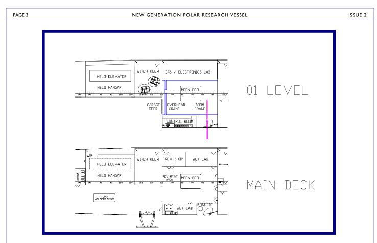
landing deck and a forward hangar had to be reconsidered. It appears that the most feasible solution was for the installation of an aft helicopter deck with a flush elevator for helicopter storage below. Sufficient space is provided such that two helicopters can be stored below on the Main Deck. This space is of sufficient size that it offers an excellent inside area for scientific vans when helicopters are not required aboard the vessel.
