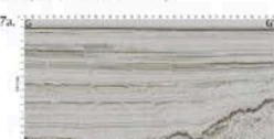
Figure 5a. Xline 788 showing Channel Surface III across compression deformation in the form of polygonal faults in the basin and grabens above the buried Pendote Ridge (Xline 10300-10350; 10310-10340).
