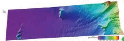
Figure 2a. 23 m MB bathymetry data. Periodic ridges in the west while troughs in the east are visible in the center and to the east. The sediment was within the distal channel have a width of 2 km with a maximum amplitude of 23 m.
