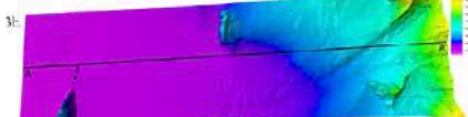
Figure 3b. 25 m emp bin 3D MCS bathymetry data. The data are plotted in two-way travel time and color-coded by depth. The data show a bright 'ridge' extending into the abyssal plain as well as a bright region to the east of the center crestal block, which is not evident in the MB backscatter data. At 50 Hz this indicates increased reflectivity deeper in the shallow sub-surface.
