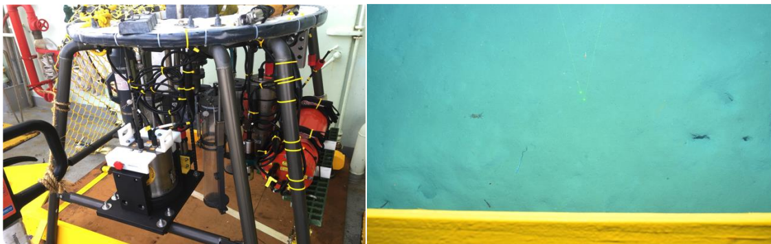
Figure 5. MISO Multicorer System (left); image of sampling area (4 m altitude; laser dots 10 cm apart)
