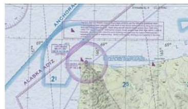
Figure 10. The ADIZ is approximately 6 nmi off the coast at Cape Lisburne Alaska.
