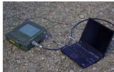
Figure 2. The CIU With Data Port Being Tapped By The Laptop Computer
