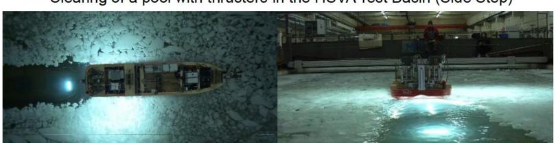
Ice Management Astern in the HSVA Test Basin (30° toe-in angle)
