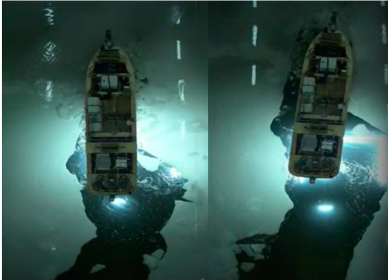
Clearing of a pool with thrusters in the HSVA Test Basin (Side Step)
