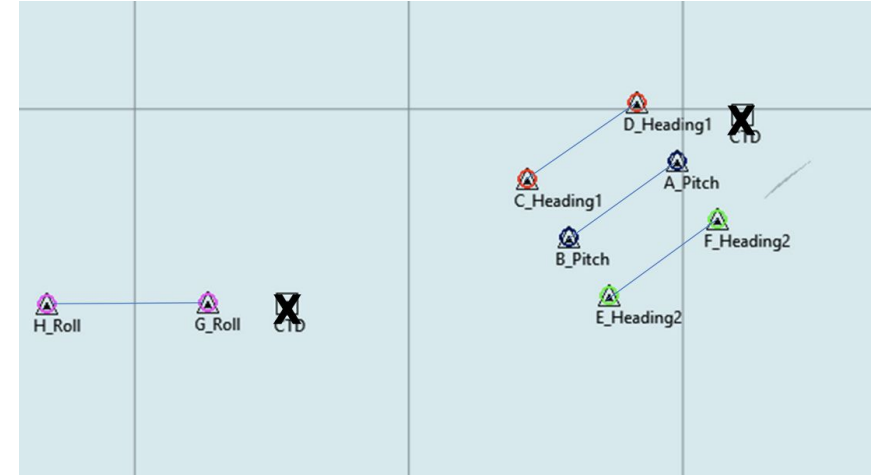
Multibeam Patch Test Track
