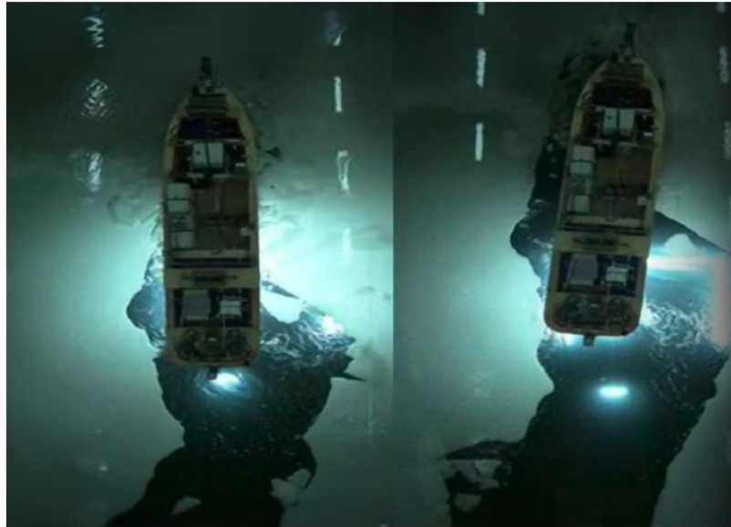
Clearing of a pool with thrusters in the HSVA Test Basin (Side Step)
