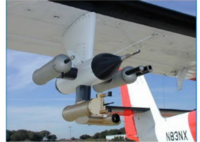
Wings: CAPS, FSSP, PCASP, CIP, PIP ... Hard points and pods for 'research' or 'guest' instruments
