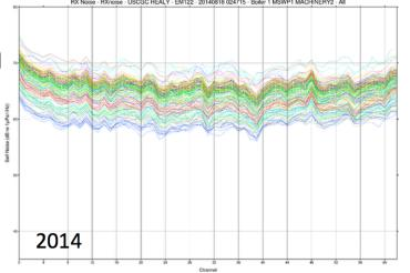
Figure 14. Noise levels perceived by the EM122 receiver under different machinery configurations. This data was collected in 2014 by Gates Acoustic. Individual test results are presented in Appendix 4.
