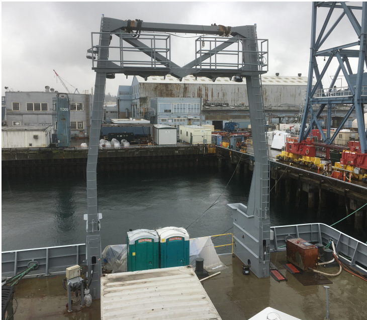
A-frame refreshed / upgraded
