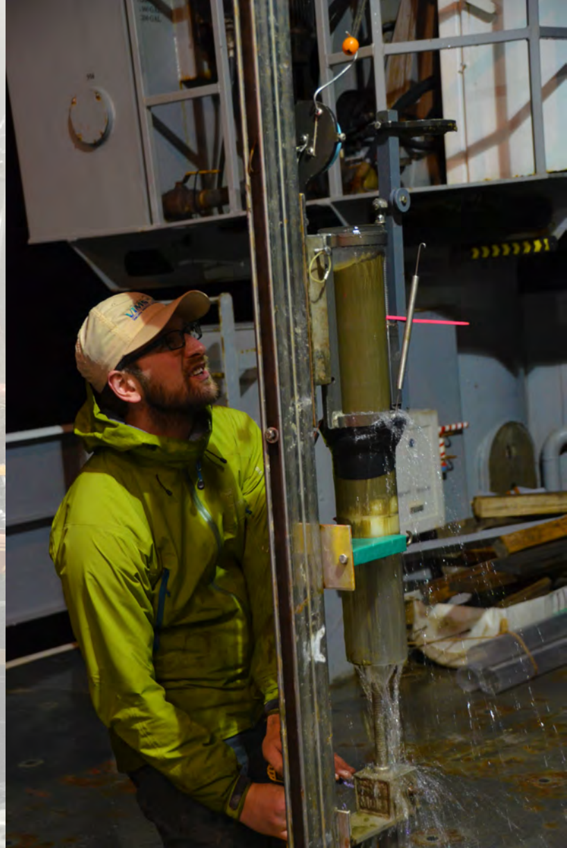
Mar. – RV Sikuliaq – Science Verification Cruise – coring - MC800 rigged with MISO 16- MP camera & strobe and depth/altimeter system and SBE25plus CTD with SBE43 O2 sensor – supported by M. Swartz - WHOI
