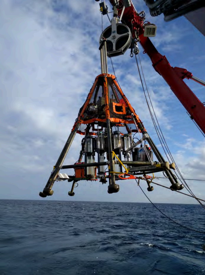
Mar. – RV Sikuliaq – Science Verification Cruise – coring - MC800 rigged with MISO 16-MP camera & strobe and depth/altimeter system and SBE25plus CTD with SBE43 O2 sensor – supported by M. Swartz - WHOI
