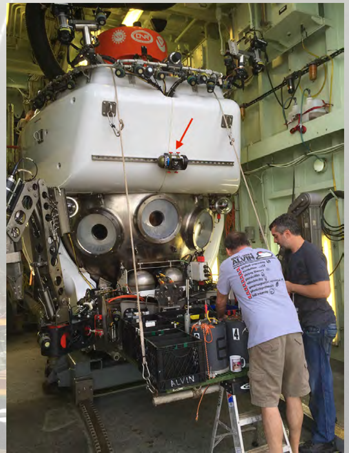
MISO GoPro 12 MP still camera mounted on Alvin
