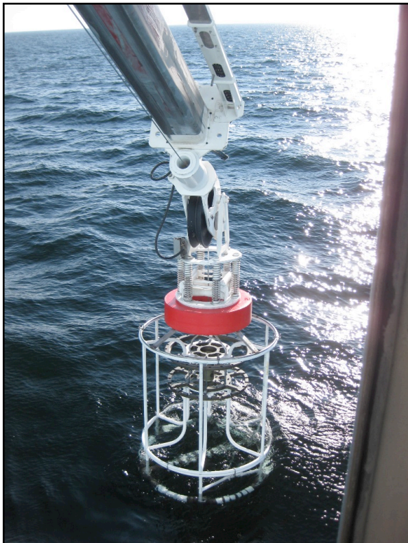
Figure 4: Boom deploying a CTD Frame.
