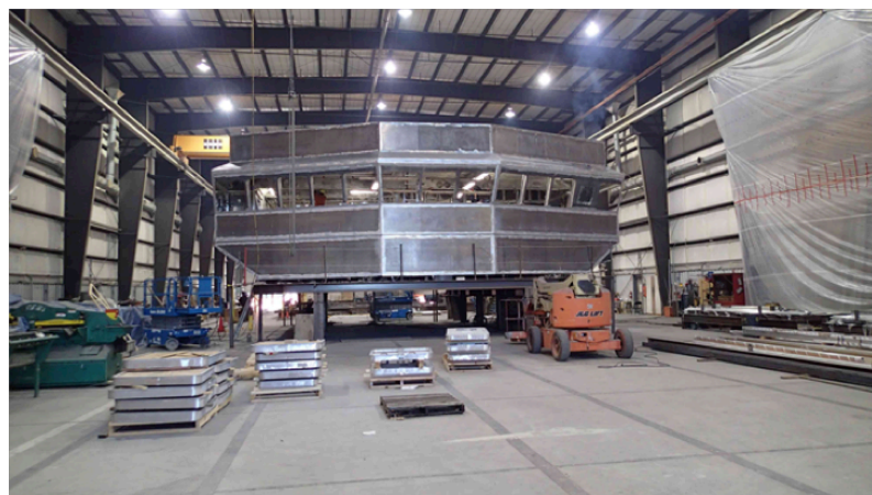
Figure 2: Sally Ride Pilot House fabrication nears completion. (photo courtesy of the Navy)
