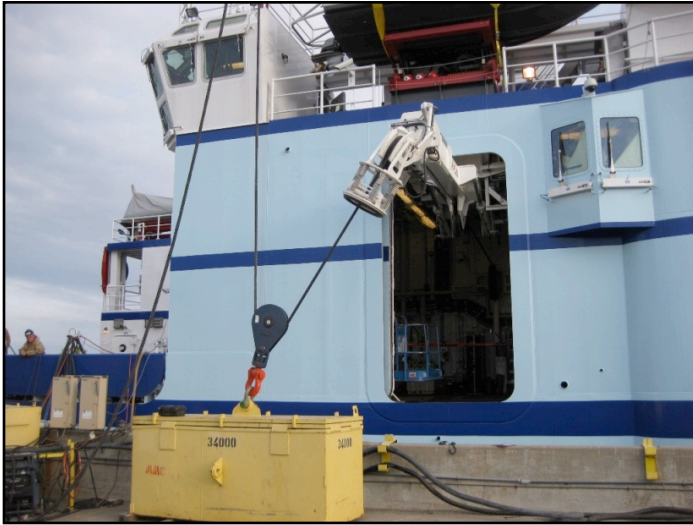
Figure 3: Boom in a tow configuration.
