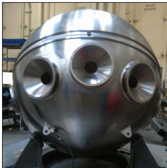
The 6500 meter personnel sphere at the fabrication facility. Note the three forward facing 7” viewports plus two 5” side viewports (photo courtesy of Southwest Research Institute)
