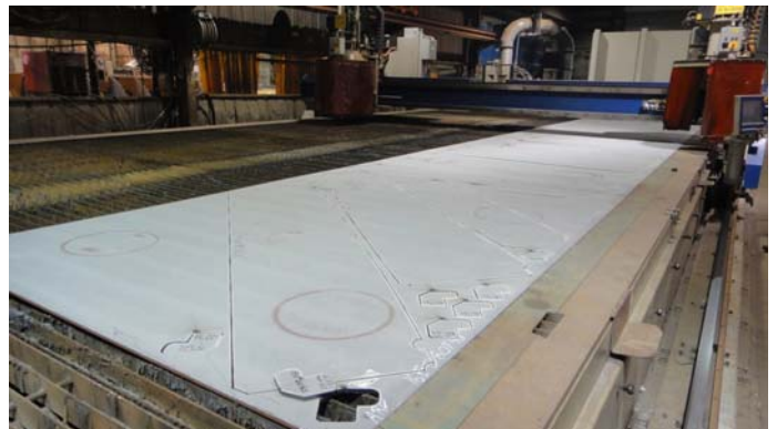
Figure 2: Steel plate is being cut using a computer controlled plasma cutting machine.
