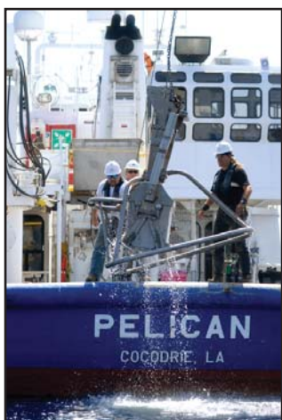
Crew lift a box core aboard the R/V Pelican in the Gulf of Mexico. The R/V Pelican spent much of 2010 conducting science in response to the Deep Horizon oil spill (photo credit: Chris Berkey).
