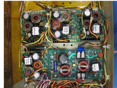
Existing DC/DC converters inside the main housing
