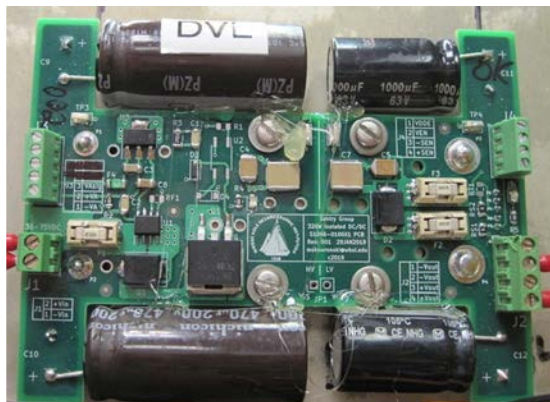
One of many replacement DC/DC converters
